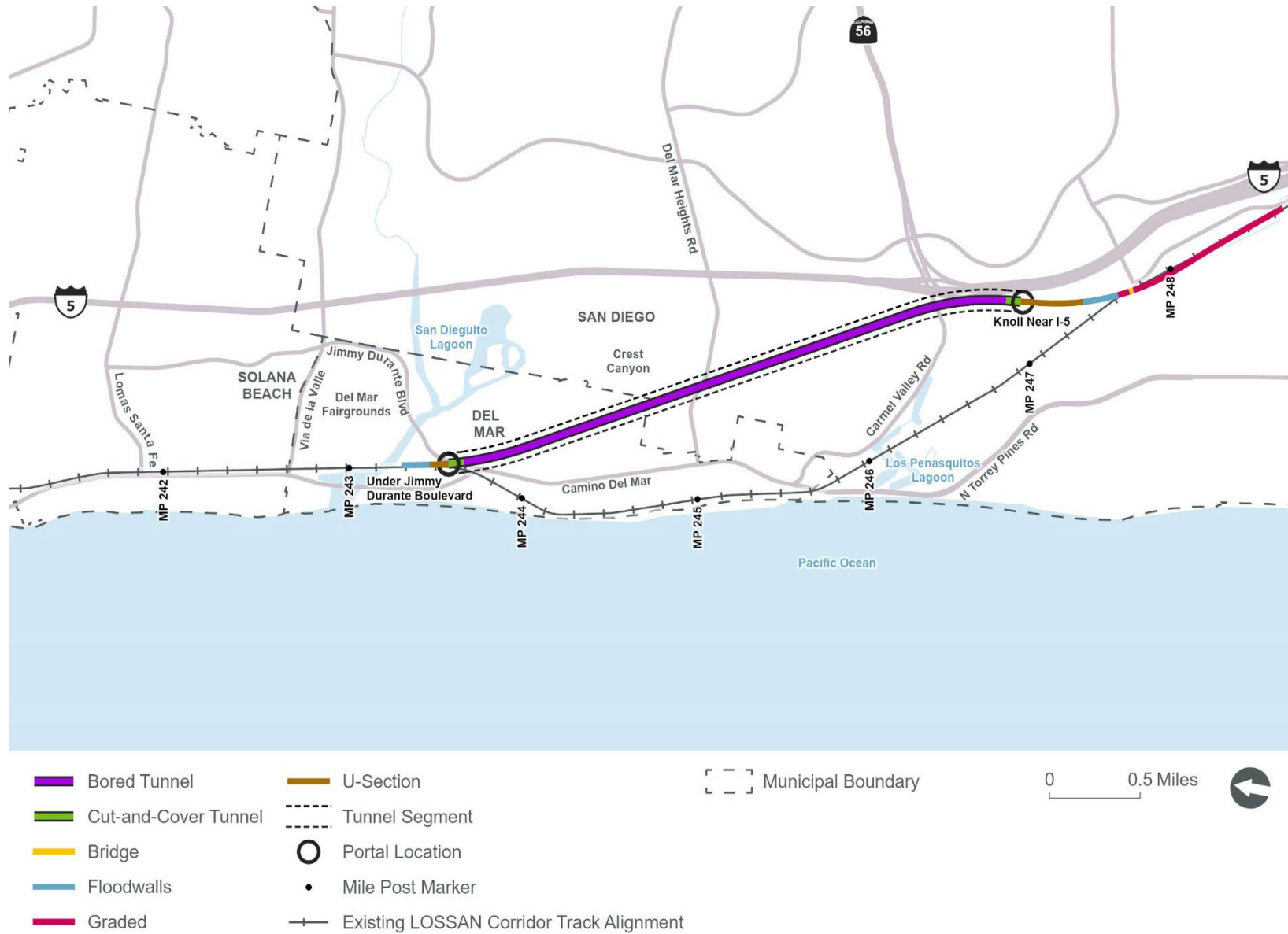
Figure 5. Alternative B Crest Canyon Alignment
